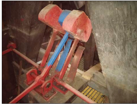
Three hammers on one bell – the 9th had a pair of carillon hammers (in red) and one of the clock's quarter chimes (in blue)
